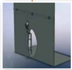
Fuel oil side penetration
